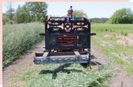
Photo 2. The crimper Ryan made using a disassembled crimper from an old haybine that they modified to fit onto the pallet forks of a tractor. For a full video of the crimper in action, visit: efao.ca/no-till-fall-broccoli-2020 .
