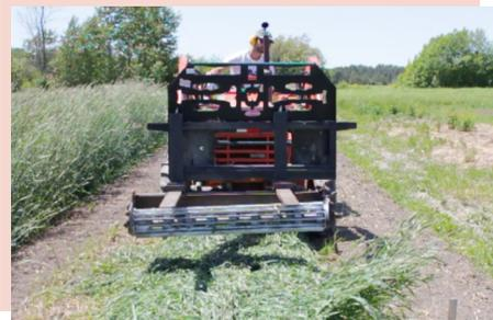
**Photo 2.** The crimper Ryan made using a disassembled crimper from an old haybine that they modified to fit onto the pallet forks of a tractor. For a full video of the crimper in action, visit: [efao.ca/no-till-fall-broccoli-2020](http://efao.ca/no-till-fall-broccoli-2020).
