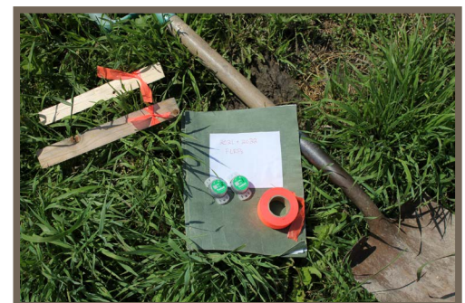
Photo 2. HOBO Pendant® MX Water Temperature Data Loggers before being buried 5 cm below the soil surface in a tilled control plot and a no-till treatment plot with landscape fabric.
